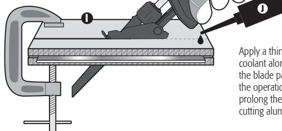
Apply a thin layer of oil or another coolant along the cutting line where the blade passes (**J**). This will make the operation easier and help prolong the life of the blade. When cutting aluminum, use kerosene.
